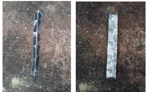
Fig.2: V-corrugated absorber plate with fins.
