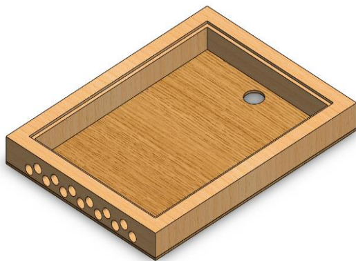
Fig.1: Wooden collector of solar air heater
