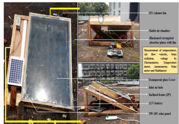
Fig.3: Indication of the isometric view of the experimental setup
